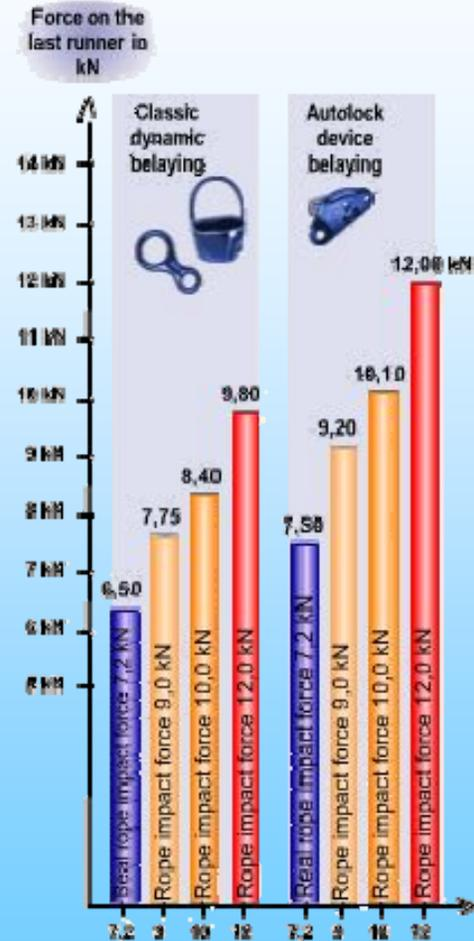
Maximum force in kN from the EN892-UIAA test written in the rope's technical notice.
